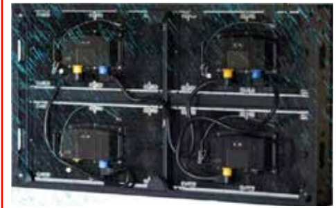
Figure 1. Sealed Solid-State LED Cabinet Architecture (Rear Interior View)
