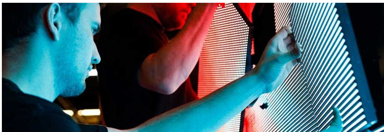
FRONT SERVICEABILITY - Technicians can access and replace display modules from the face of the sign without requiring rear cabinet access.
