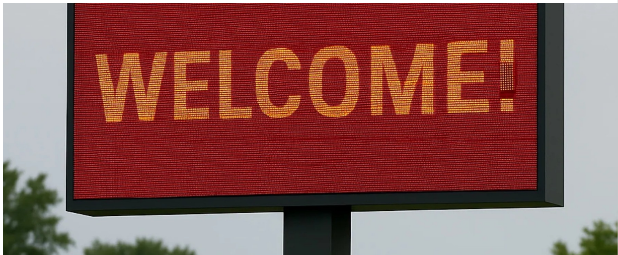
MISMATCHED COLOR - Replacement modules that do not match can leave visible patches even when the sign technically operates.
